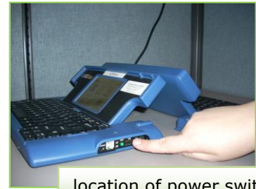
location of power switch
